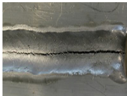
POROSITY: Aluminum Fillet Weld CRACKED: Aluminum Fillet Weld UNDERFILL: Aluminum Fillet Weld
