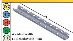
Used to support mesh system without the use of guides & clamps
