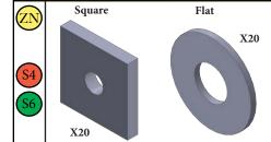
Used to distribute large loads and act as a shim when securing fixtures
